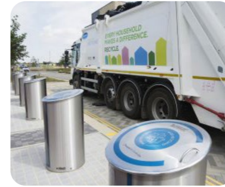
Eddington, Cambridge Underground chutes replace thousands of traditional wheelie bins in an innovative waste disposal system.
